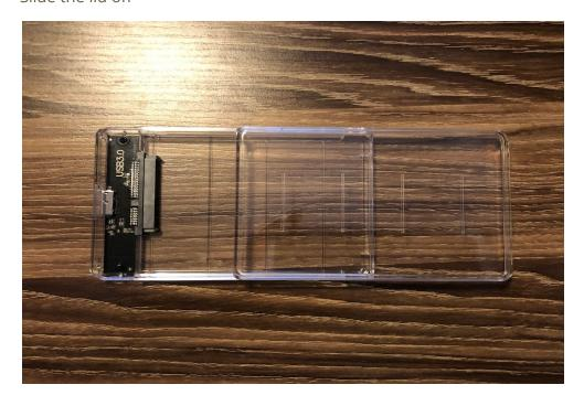
Insert the hard drive and slide the lid back on
